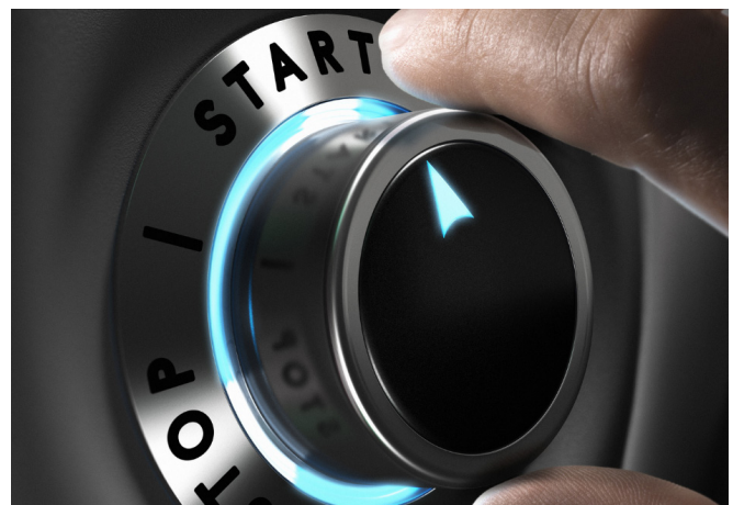
Figure 3: Bivar's LED light guides integrate the LED, lens, and PCB with microcontroller in a single housing. The large-area devices are available in multiple form factors, including annular (shown here), rectangular, and "bar graph."
